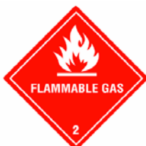
HSNO Class 2.1.1A flammable gases (UN Class 2.1) HSNO Class 2.1.2A: flammable aerosols (UN Class 2.1)
